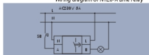
Wiring diagram of NTE8-A time relay
